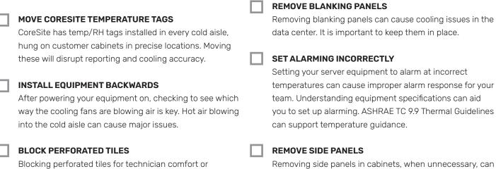
Blocking perforated tiles for technician comfort or with boxes can cause cooling issues in the space. A consequence could be temperature issues in your racks or energy overuse.
